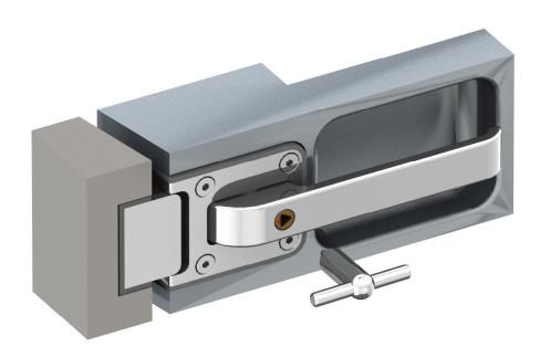
The Structor lock type 330 is primarily designed for use in bulwark doors on board of luxury yachts. It has a weldable aluminium housing that leaves the door body airtight. This lock is available for inward and outward opening doors. Picture above shows an optional child lock operated with a separate key. A push button childlock can also be supplied.
